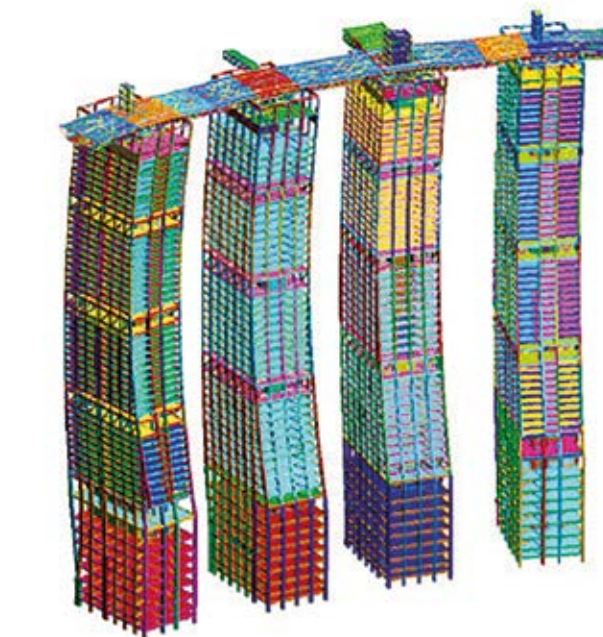
LS-DYNA model to analyse interactions between the conservatory and the towers during earthquakes
